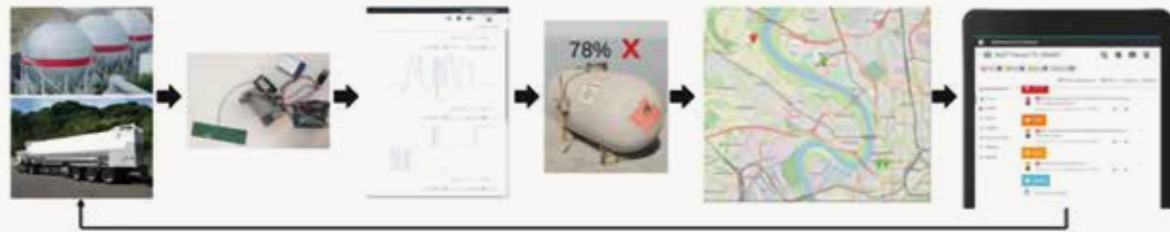
Fig. 18: The digital twin of the hydrogen vessel in action
