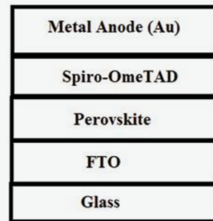
Fig. 33: (e) Schematic of ETL-free perovskite configuration.
