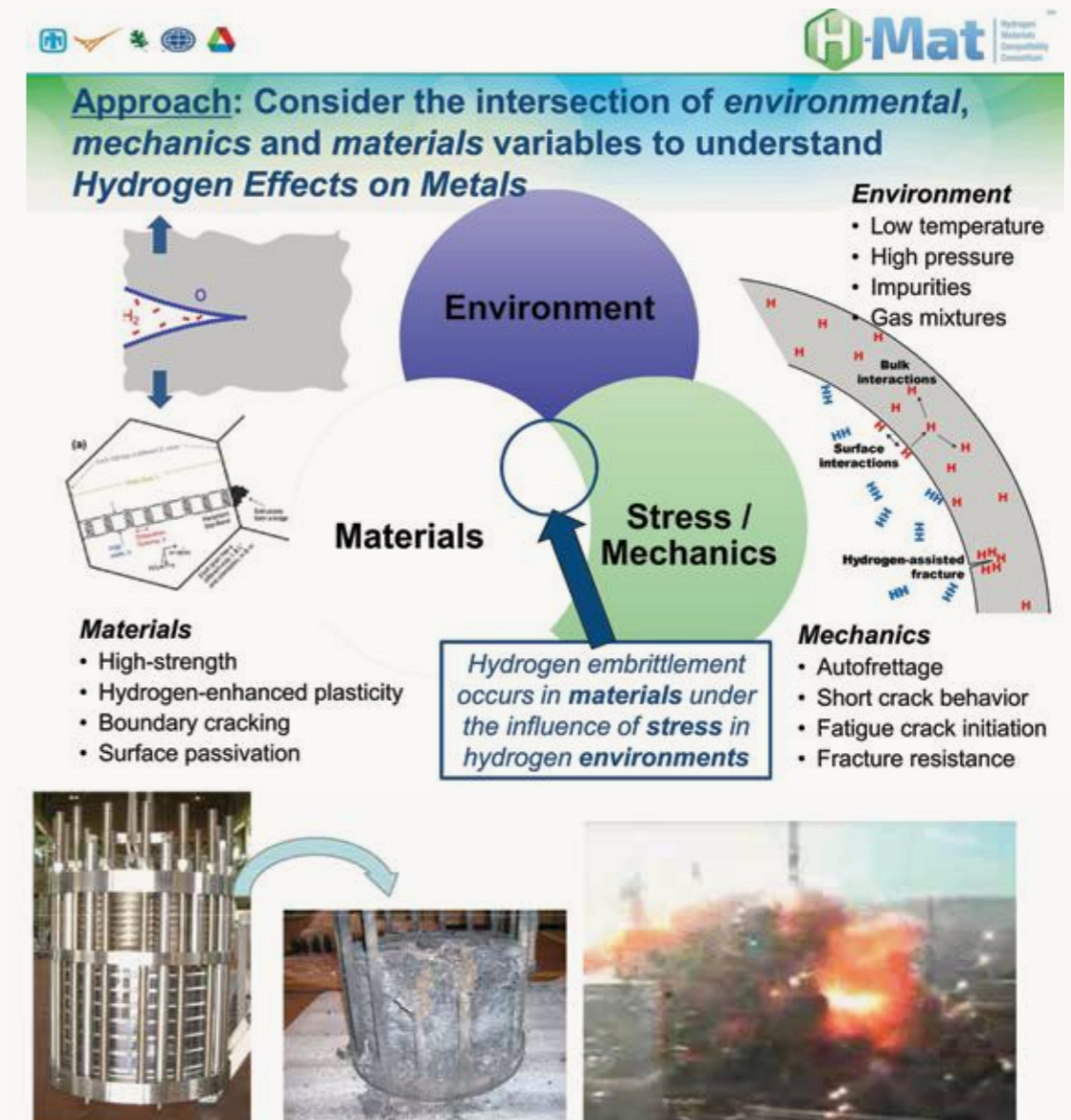
Fig. 22(a): Titanium electrolyser before and after the accident ( https://hyresponder.eu/wp-content/uploads/2021/04/Lecture-1-slides.pdf )
