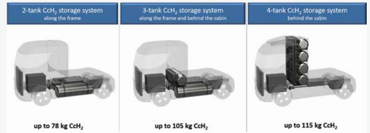
Fig. 4: CRYOGAS onboard storage allows up to 40 kg of hydrogen being stored in one vessel. A two-vessel package allows storing up to 80 kg in a typical truck platform, sufficient to reach a 1,000 km range. Three-vessel packages or more enable even higher ranges and energy supply in special heavy-duty applications.
