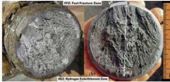
Fig. 22(b): Fracture face of Hot dip galvanized (HDG) high strength steel anchor rods https://link.springer.com/article/10.1007/s11668-017-0250-2
