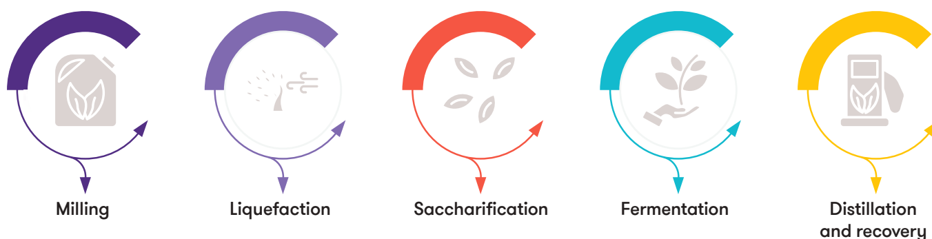
Figure 3: Processes involved in dry grind method of ethanol production
